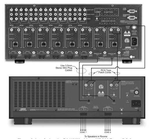
Figure 8: Interfacing the PA4100X with an MRC88 Zones 7 & 8
